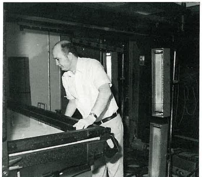
Jerry Heffington operates the overhead camera used for film negatives and halftones.
