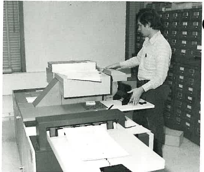
The Aperture card 35 millimeter microfilm printer is used to make larger copies from the microfilm cards.
